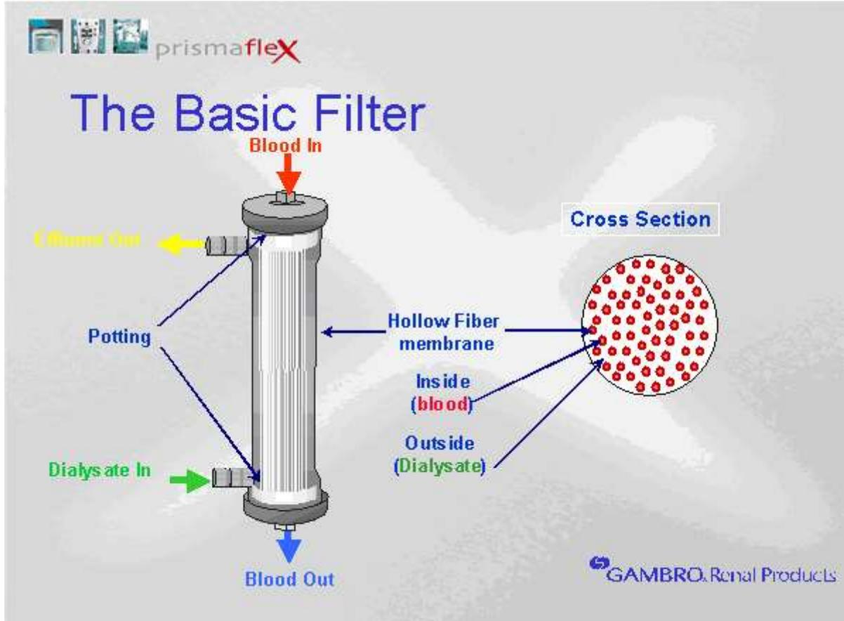
Fig. 19. The filter function (Gambro, 2013)
